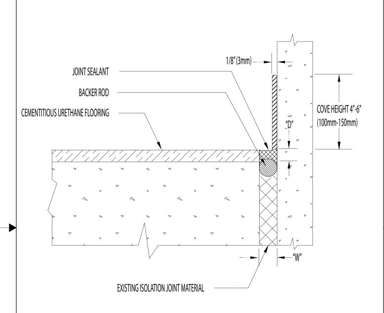
D = W /2 D = DEPTH OF BACKER ROD W = WIDTH OF JOINT
