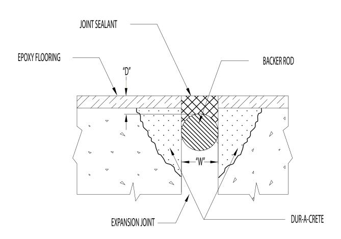
D = W/2 D = DEPTH OF BACKER ROD W = WIDTH OF EXPANSION JOINT
